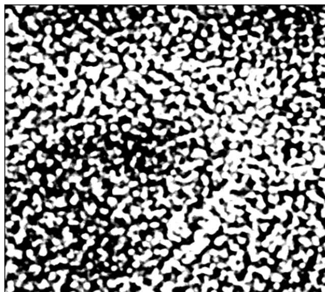
Figure 7. Typical morphology for SAN/PMMA 50/50 blend at 164 °C observed by optical microscopy.
